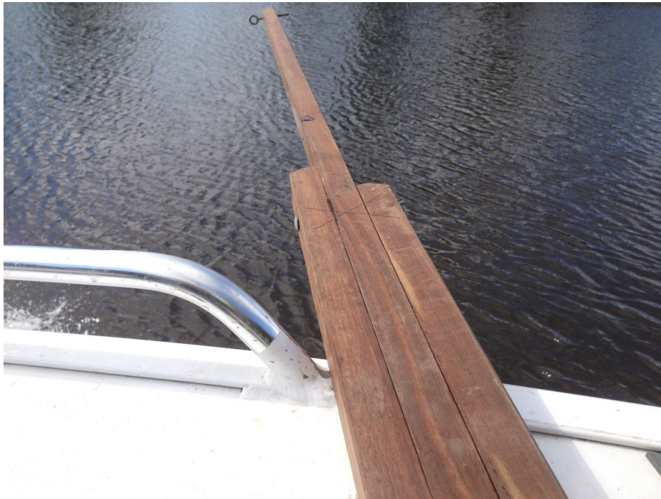
Photos 3 & 4: deployment boom mounted across front of the boat anchored on the opposite side.
